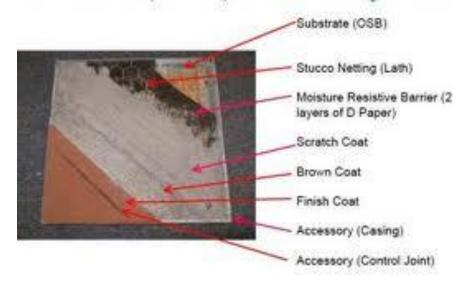
Installed over wood- planking, solid sheathing- plywood, OSB, or insulated sheathing
